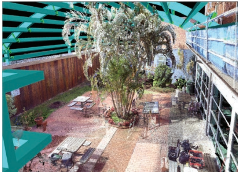
3D scan of an external eating area at Ipswich hospital. Shown with the proposed roof structure 3D model overlaid.
